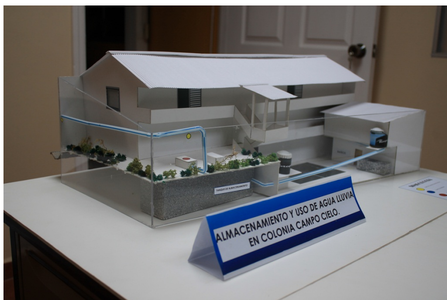
Image 2 – Model of rainwater harvesting model at the individual level, as an adaptation strategy to reduce water infiltration on steep slopes, prevent landslides, and increase water supply
